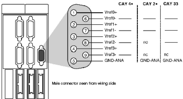
**Connection of Counting Signals****Connectors Pinouts**
