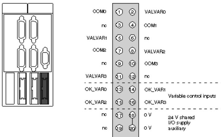
COMx – VALVARx: potential free contact to validate variable speed controller
